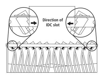
Figure 5. IDC slot position.
